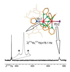
The reaction of the potassium salt of bulky dipyridylamine with  $[YbI_2(thf)_4]$  or with  $[EuI_2(thf)_4]$  afforded novel dinuclear  $Yb^{II}$  and  $Eu^{II}$  complexes which were structurally characterized by  $^{171}Yb$  NMR and  $^{151}Eu$  Mössbauer spectroscopy. The ligand is highly flexible in its coordination behavior and a variety of bimetallic Yb complexes were isolated and characterized.
